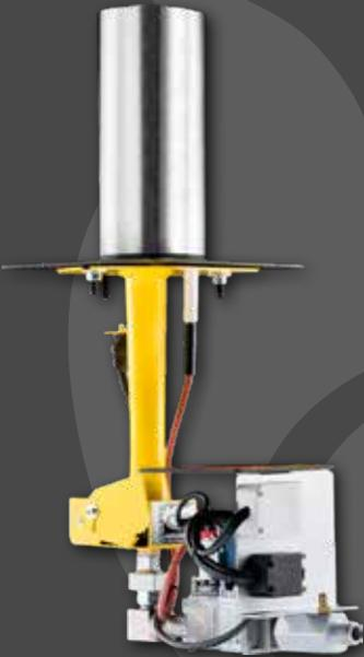
**DRAGO D1/S** is a professional burner specifically designed to heat rotating oven floors. This model is equipped with an electronic burner control device and a gas control with automatic shut-off valves and full electrical modulation. It comes with a simple ON/OFF control panel that is exclusive to this burner model.
